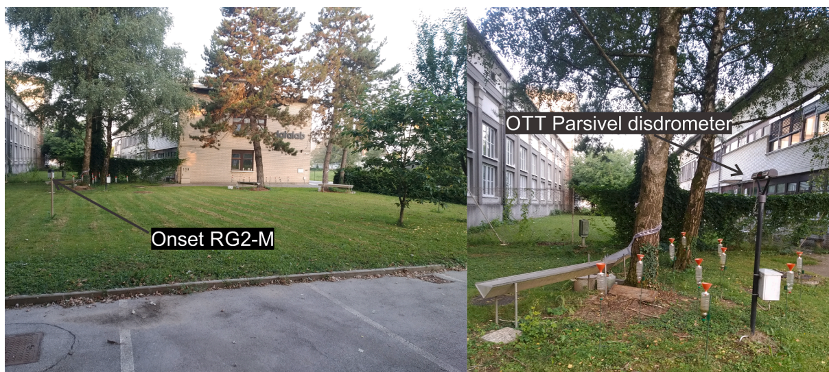
Fig. 1. Photo of the study area, left photo shows the entire plot, while the right photo shows the measuring equipment below the birch canopy. The disdrometer positioned above the canopy is set-up on the building on the left side of the photo, around 50 m from the disdrometer below the canopy.
