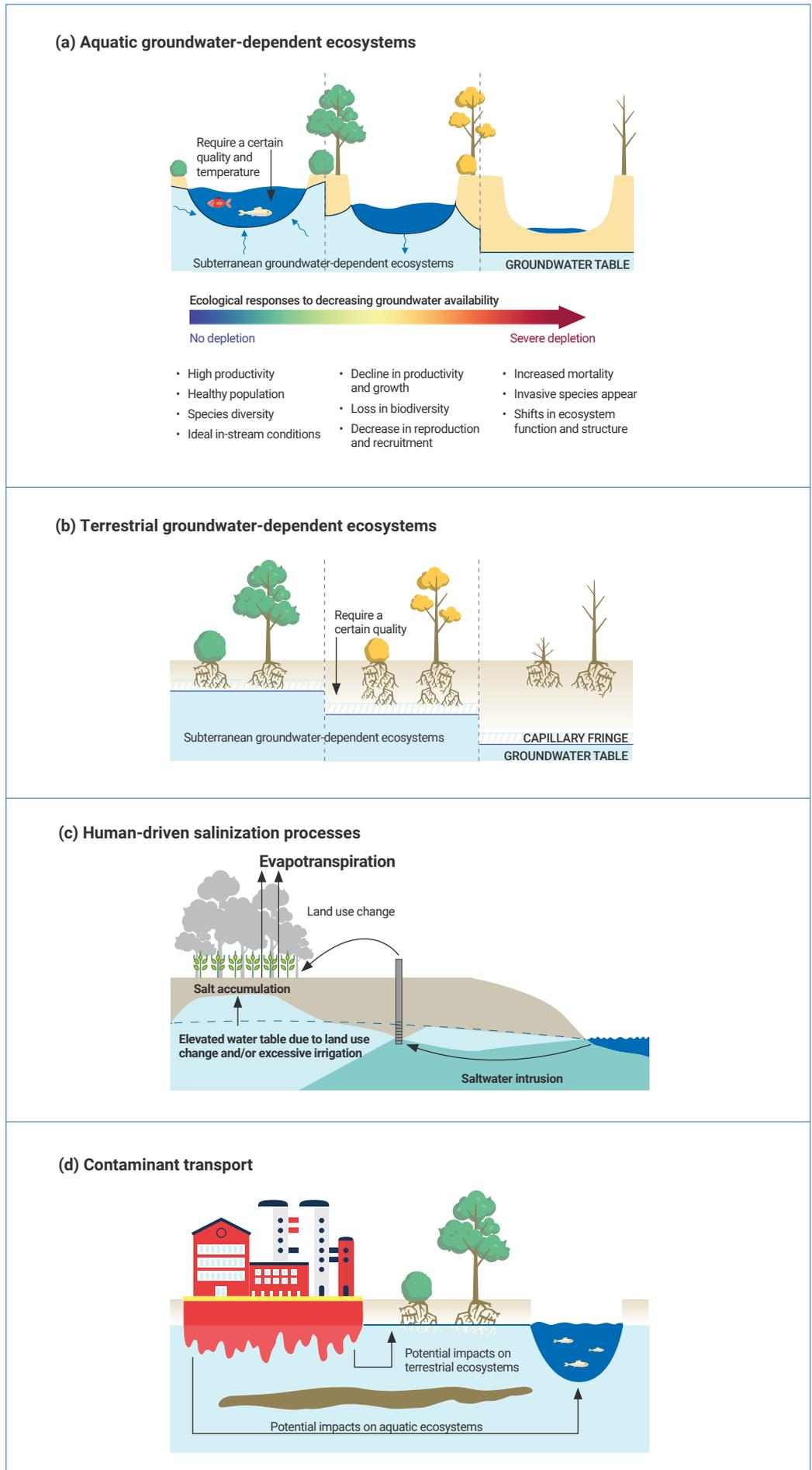
Note: (a) and (b) ecological responses to decreasing groundwater availability: (a) aquatic and (b) terrestrial groundwater-dependent ecosystems; (c) and (d) water quality and contamination impacts on groundwater-dependent ecosystems: (c) soil and groundwater salinization processes due to land use change, coastal pumping and irrigation, and (d) local and regional impacts of contamination events due to regional groundwater flow systems.
