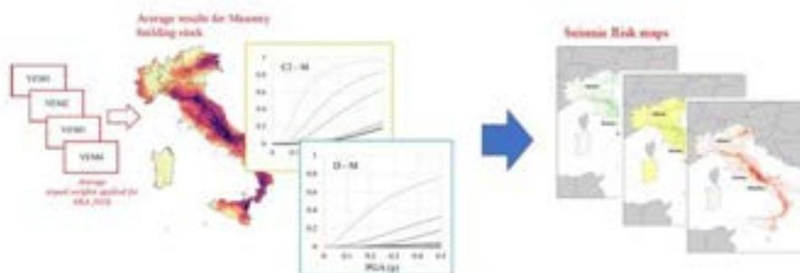
**Figure 3.3:** An example of the results combination process: the output of models for masonry (VEM1 to VEM4) are weighted to obtain the risk maps in terms of damaged dwelling (adapted from Dolce et al. 2021).
