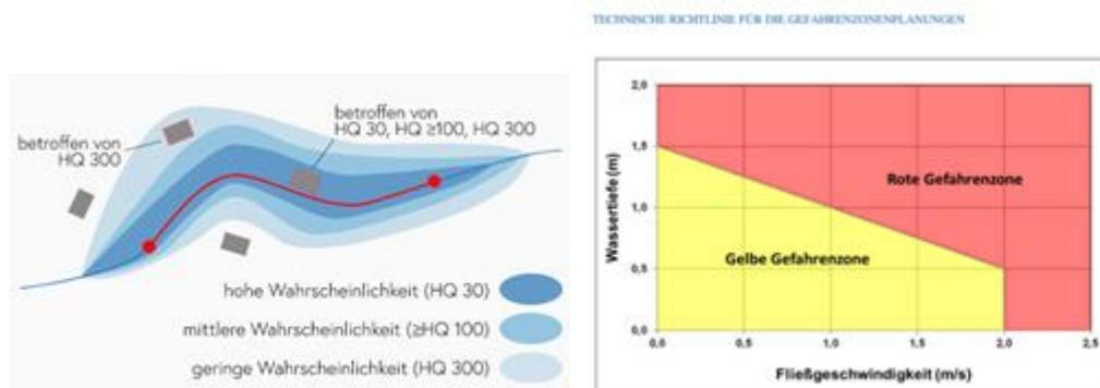
**Figure 4.7:** left: Austria used three flood scenarios to assess the individual hazard/risk (source BMLRT, 2018); right: Classification of hazard zones due to the interaction of the water depths (m) and flow velocities (m/s) (energy line) (BMLRT, 2018b).
