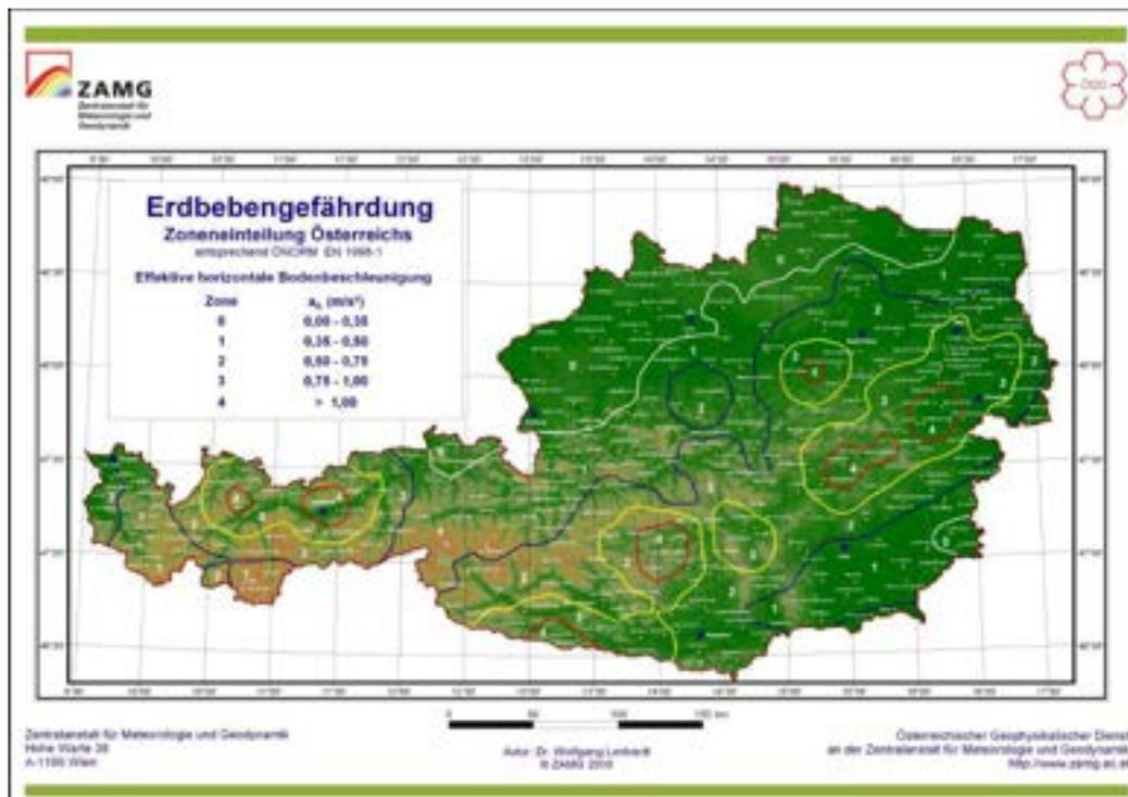
**Figure 4.3:** The seismic hazard map of Austria that is included in the current ÖNORM 1998-1 outlines the seismic zones and the “effective” ground acceleration in m/s<sup>2</sup> (which is considered to be 70% of the maximum ground acceleration (source: ZAMG, s.a. ©ZAMG 2010).
