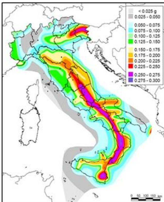
**Figure 3.1:** Seismic hazard map of Italy expressed in terms of horizontal peak ground acceleration for soil type A with a probability of exceedance of 10% in 50 years, referring to stiff soils ([www.ingv.it](http://www.ingv.it)).
