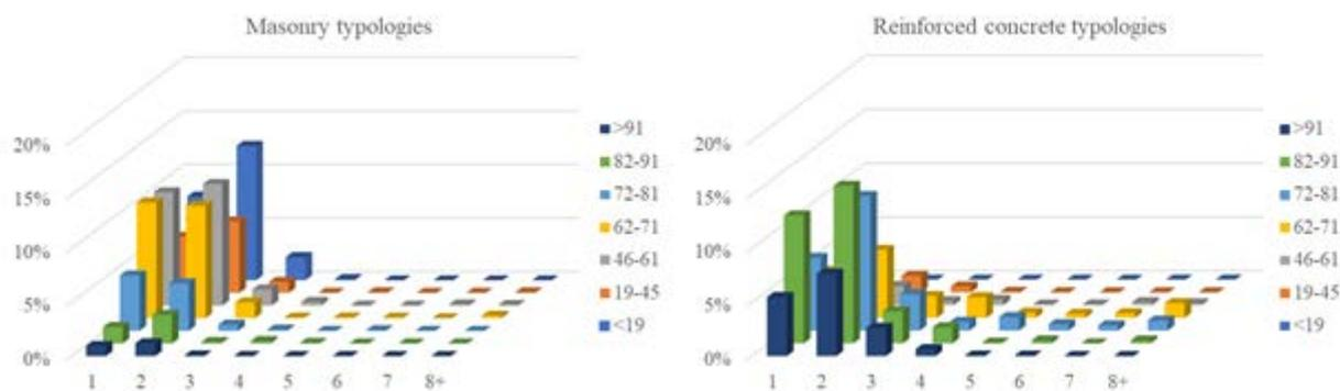
**Figure 3.2:** Proportion of masonry and reinforced concrete typologies in terms of construction age and storey number for the town Angri, identified according to ISTAT 2001 database.
